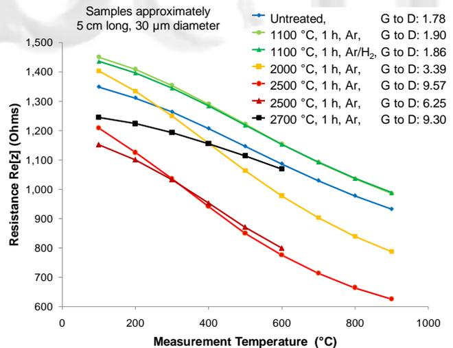
Fig. 1. Resistance versus temperature of CNT yarn previously annealed in various environments
