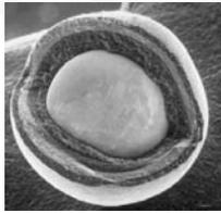
**Figure 1:** Exemple of TRISO HTR fuel particle. The layers are, from the kernel out: porous pyrocarbon (buffer), inner dense pyrocarbon (IPyC), SiC, outer dense pyrocarbon (OPyC).
