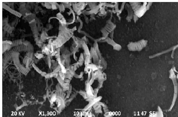
**Fig. 4** Coned nanocoil and nanoribbon.
