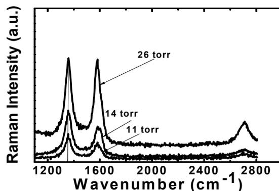
Fig. 2 Effect of gas pressure on the quality of carbon nanotubes.
