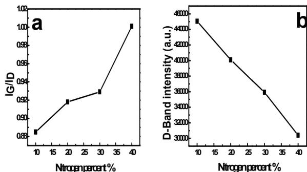
**Fig. 3** Effect of nitrogen addition on the CNTs a) relation between the ratio  $I_G/I_D$  and the nitrogen portion, b) Relation between the nitrogen portion and the D-band intensity.
