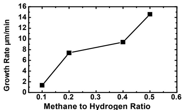
Fig. 1 Effect of the ratio between methane and hydrogen on the growth rate of the CNTs.
