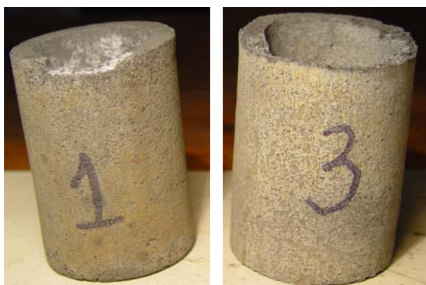
Fig.3 Experimental carbonaceous metalcarbide crucibles during testing.
