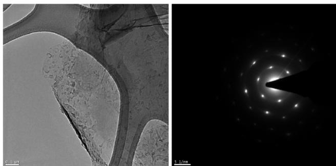
**Fig. 2.** TEM micrograph of a GNR and SAED pattern
