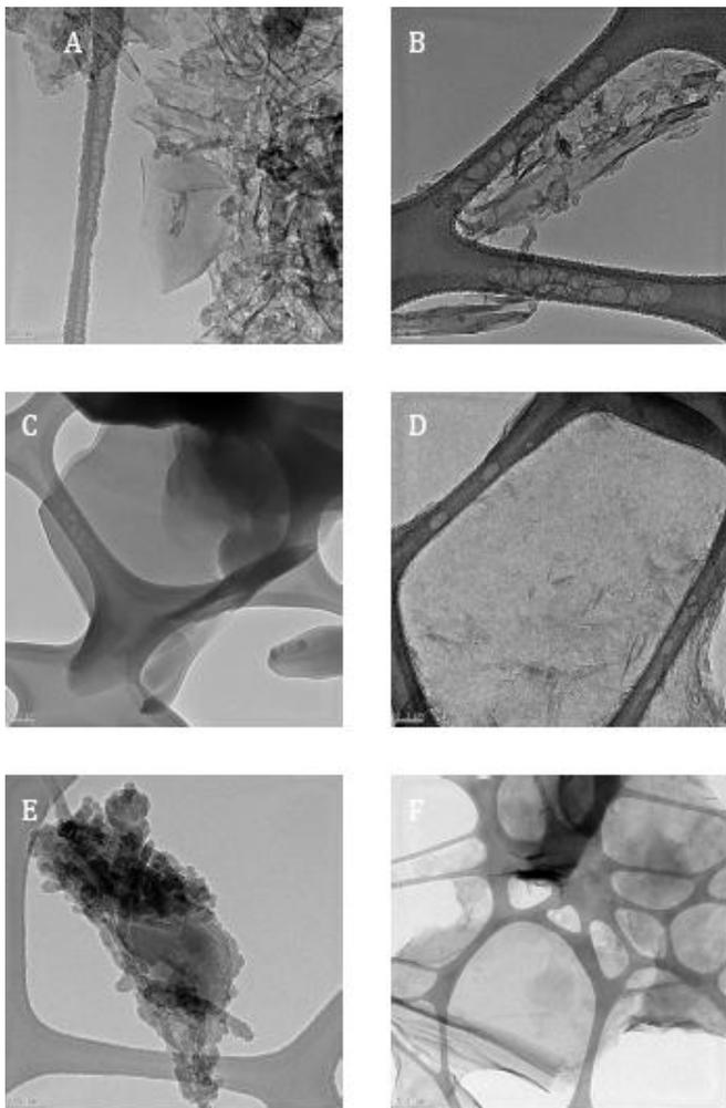
**Fig. 1.** TEM micrographs of GANF 100 wt-% oxidized (A), GANF 200 wt-% oxidized (B), GANF 400 wt-% oxidized (C), GANF 500 wt-% oxidized (D), CNT 500 wt-% oxidized (E) and graphite 400 wt-% oxidized
