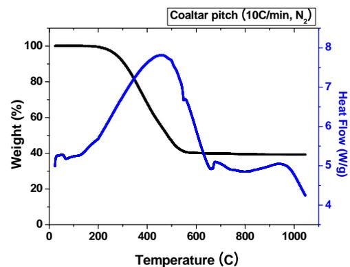
Fig. 1. Results of thermal analysis of coal-tar pitch
