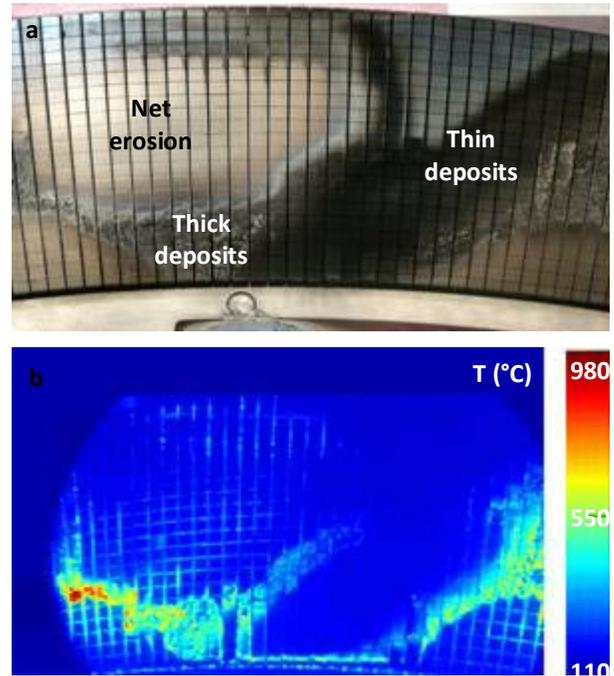
**Fig. 1** Dismantled part of the toroidal limiter: (a) erosion- or deposition-dominated zones, and (b) temperature cartography obtained by infrared thermography.
