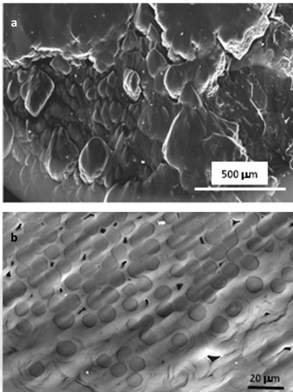
**Fig. 2** SEM images of the top surface of (a) a thick deposit tile and (b) an eroded tile.
