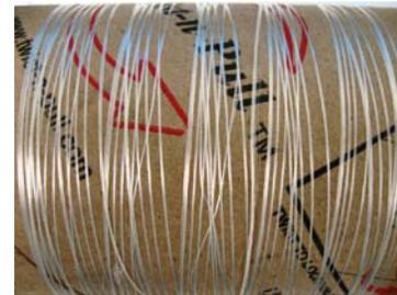
**Fig. 3** Close up of 100 two PAN precursor fiber traverse-wound on a 3" cardboard core
