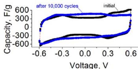
**Fig. 1.** Cyclic voltammetry of a carbon-polymer composite electrode tested in a symmetric two-electrode configuration before and after 10,000 charge-discharge cycles.
