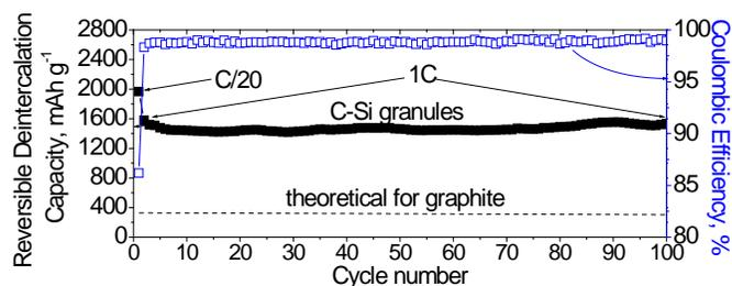
**Fig. 2.** Reversible Li deintercalation capacity and coulombic efficiency of the C-Si granule electrode vs. cycle number in comparison to the theoretical capacity of graphite [6].
