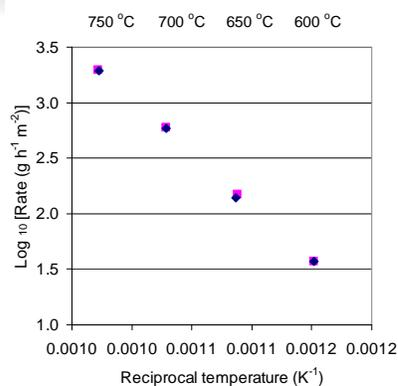
**Fig. 4:** Arrhenius plots of oxidation rates
