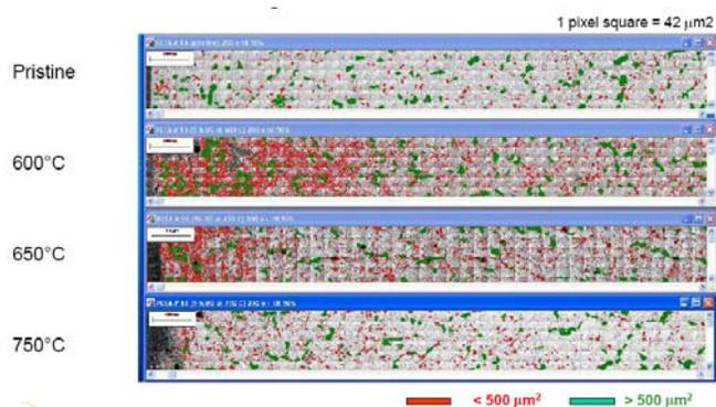
**Fig. 3:** Progress of oxidized layer with temperature (5 % net weight loss). Mosaic images cover the radius of specimens from surface (left) to center (right). Scale bar = 1 mm.
