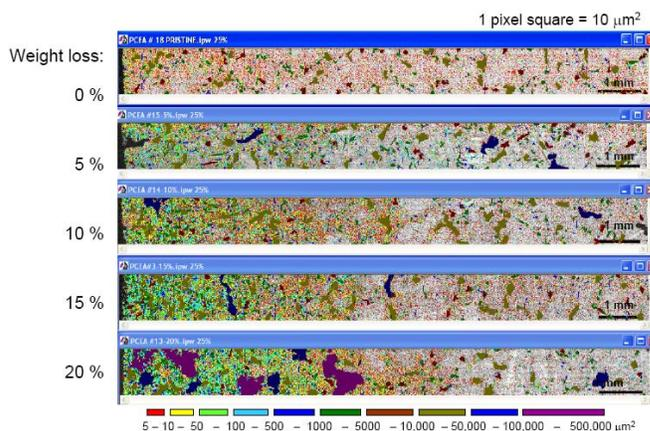
**Fig. 5:** Development of porosity in the oxidized layer with the level of weight loss at 600 °C. Scale bar = 1 mm.
