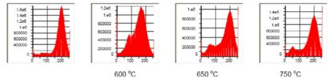
**Fig. 1:** Intensity histograms of pristine and oxidized graphite specimens (20 % weight loss at various temperatures).
