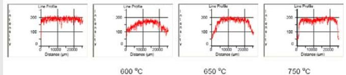
**Fig. 2:** Profile analysis of pixel intensity distribution along a specimen's diameter (25.4 mm) for pristine and oxidized graphite (20% weight loss at various temperatures).
