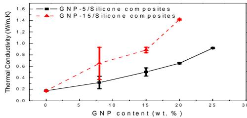
**Fig. 3.** Thermal conductivity of GNP/silicone composites produced by SM as a function of wt.% of GNP
