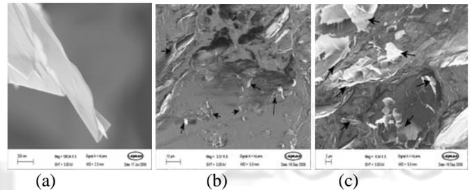
Fig. 2. SEM images of (a) GNP, (b) 20 wt.% GNP-5/silicone and (c) 20 wt.% GNP-15/silicone composites produced by SM (arrows pointing towards some of the GNP in the silicone matrix)
