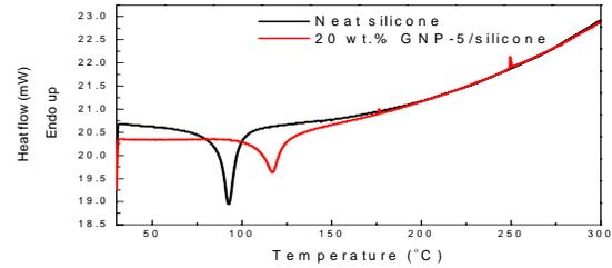
Fig. 1. DSC scans of neat silicone and GNP/silicone dispersion
