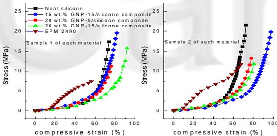
**Fig. 4.** Two replicate compressive stress-strain curve sets for neat silicone, EPM2490, GNP-5/silicone and GNP-15/silicone composites
