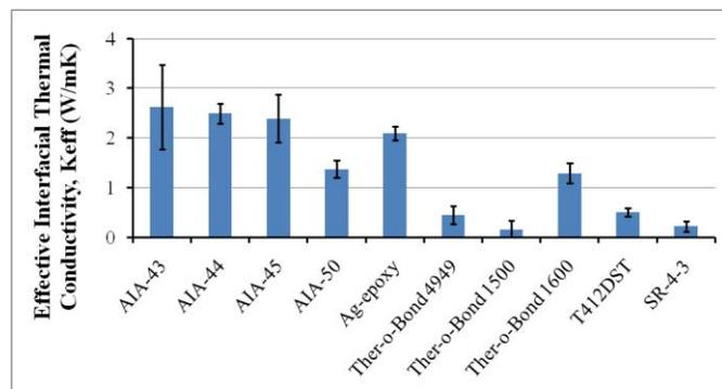
**Fig. 2** Effective interfacial thermal conductivity of sandwich assemblies
