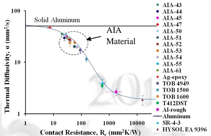
**Fig. 1** Thermal properties of interface materials bonding mill-finish Al substrates.
