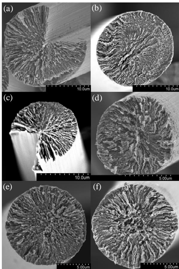
**Fig. 2** SEM images of (a) 0wt% and (b) 0.3 wt% SAR MWCNT A-series carbon fibers, and (c) 0wt% (d) 0.1 wt% SAR MWCNT (e) 0.3 wt% BN and (f) 0.3 wt% CB B-series carbon fibers.
