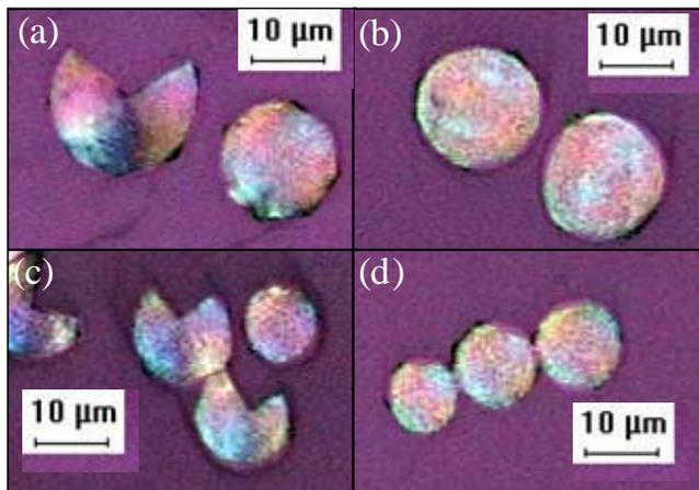
**Fig. 1** Optical micrographs of (a) A-series 0 wt% (b) A-series 0.3 wt% SAR MWCNT, (c) B-series 0 wt% (d) 0.1 wt% SAR MWCNT.
