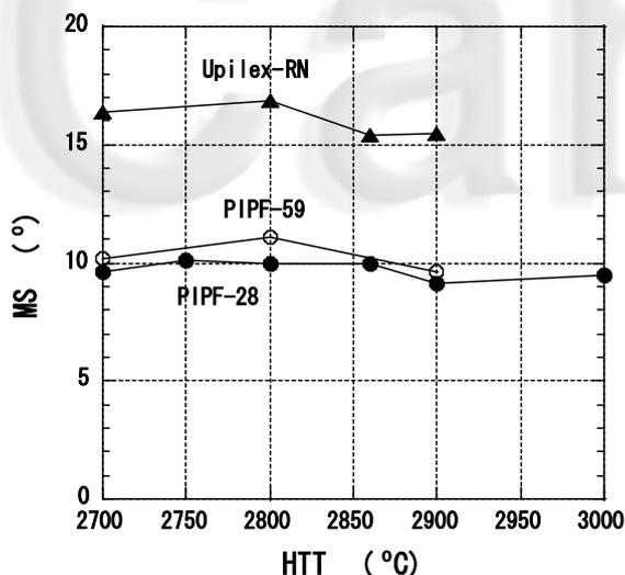
**Fig. 4** MS as a function of HTT for PIPF-28, PIPF-59 and Upilex-RN heat-treated for 1 min at each HTT except 3000°C-treated PIPF-28 (30 min).
