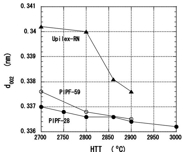
**Fig. 3**  $d_{002}$  as a function of heat treatment temperature HTT for PIPF-28, PIPF-59 and Upilex-RN heat treated for 1 min at each HTT except 3000°C-treated PIPF-28 (30 min).
