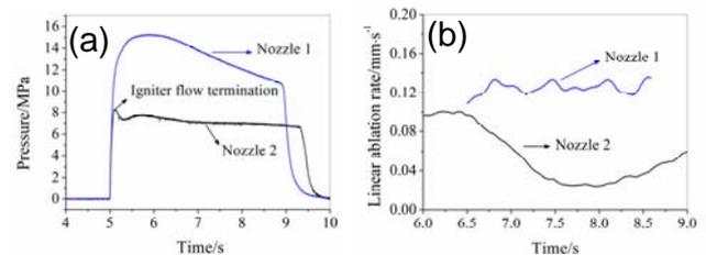
Fig. 2 (a) Recorded pressure-time traces, (b) linear ablation rate of nozzle throat.
