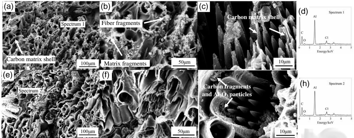
Fig. 3 Morphology and EDS patterns of C/C composite throat: (a-d) Nozzle 1, (e-h) Nozzle 2.
