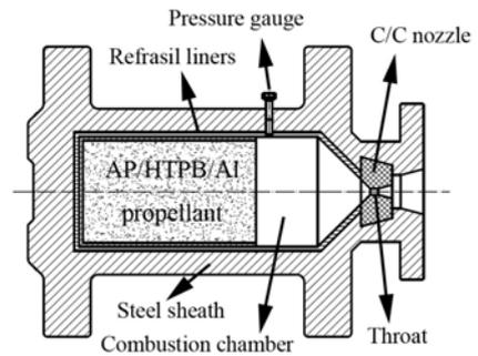
Fig. 1 Schematic of the small SRM hot-fire testing system.
