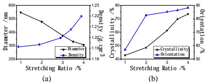
**Fig. 3** Effect of stretching on (a) diameter and density, (b) crystallinity and orientation of PAN nanofiber bundles
