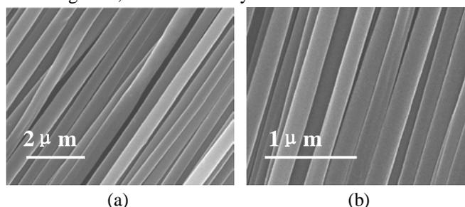
**Fig. 2** SEM images showing the representative morphologies of the electrospun PAN nanofiber bundles (a) before and (b) after stretching
