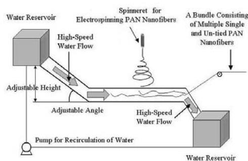
**Fig. 1** Schematic representation of the electrospinning setup for preparing continuous and uniaxially aligned nanofibers
