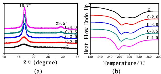
**Fig. 4** (a) XRD and (b) DSC curves of as-electrospun PAN nanofiber bundles (C) and nanofibers with different stretching ratios, such as 2.0,3.0,3.5,4.0
