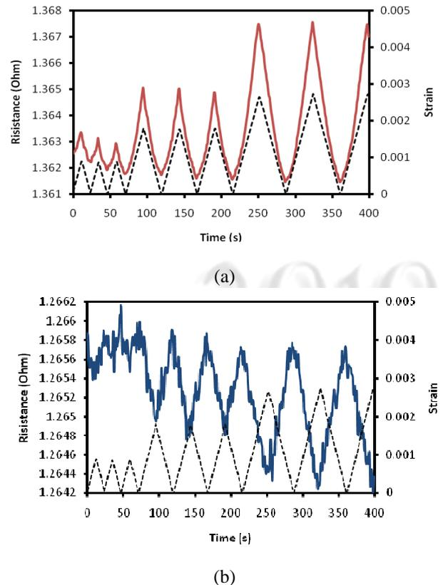
**Fig. 1** Strain sensing characteristics of a one-lamina carbon fiber epoxy-matrix composite sensor attached to a solid in the form of a 22-lamina glass fiber epoxy-matrix composite. The resistance is obtained during repeated flexural loading at progressively higher strain amplitudes up to 0.003. The resistance is shown by solid curves. The flexural strain is shown by dashed curves. (a) Tension surface. (b) Compression surface.
