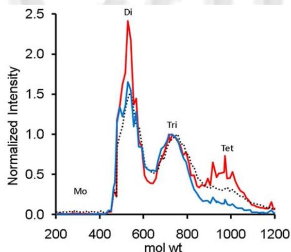
**Figure 3.** MALDI spectra of trimer-rich bottom products. Trimer A from Col-2 at  $+\Delta T$  (380-380-350-350 °C), S/P = 17/1, 60 bar (—), Trimer B from Col-2 at  $+\Delta T$  (400-400-350-350 °C), S/P = 17/1, 63 bar (—), and Trimer C from Col-1 at  $+\Delta T_2$ , S/P = 12.1/1, 69.9 bar (••••). Spectra have been normalized to trimer content (max peak height = 1) to facilitate comparison.
