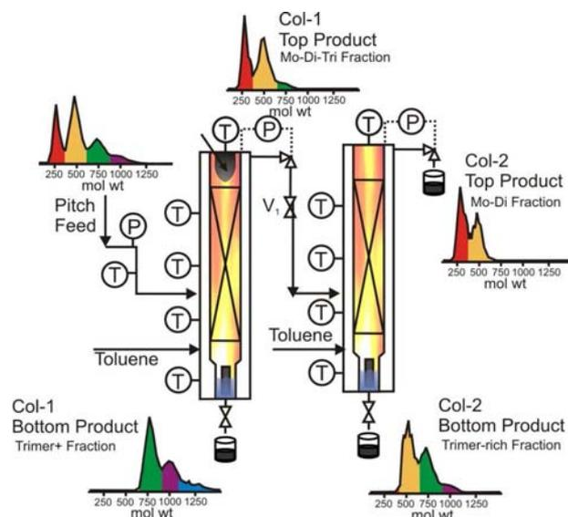
**Figure 1.** Fractionation of M-50 via two-column DGE to produce mesophase pitches. Spectra shown are actual MALDI spectra of feed pitch M-50 and extraction products obtained in this study
