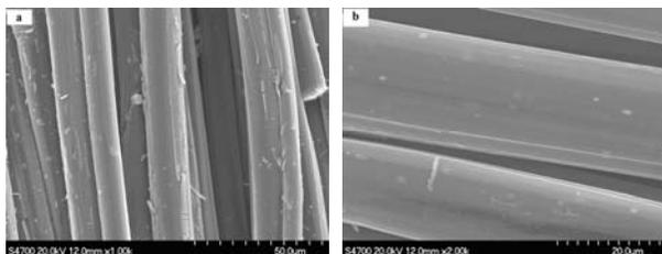
Fig. 4 SEM of carbon plate before and after titanium catalytic graphitization (a: before graphitization; b: after graphitization)
