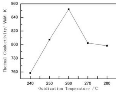
Fig. 1 Thermal conductivity of the carbon plate of different oxidation temperature
