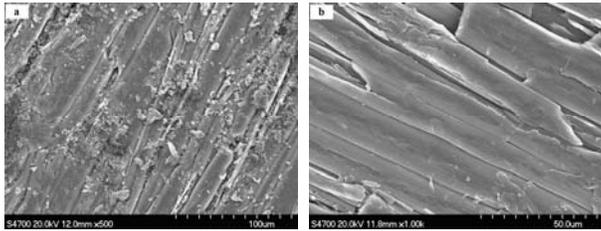
Fig 2 SEM of carbon plate before and after boron catalytic (a: before graphitization; b: after graphitization)
