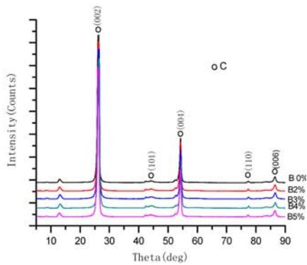
Fig 3 XRD of Boron Catalytic graphitized Carbon Plate
