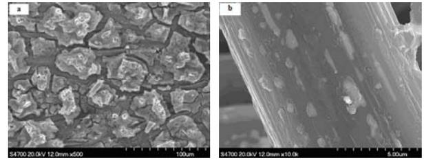
Fig. 5 SEM of carbon plate before and after Ti-B catalytic graphitization (a: before; b: after)
