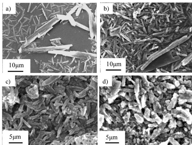
**Fig. 1** The SEM observation results of the crystalline C<sub>60</sub> particles with the droplets per discharge and the total droplets of (a) 10 and 200, (b) 10 and 400, (c) 15 and 300, and (d) 40 and 800, respectively.
