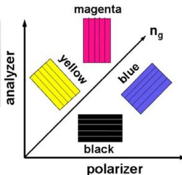
**Fig. 2** The relation between colors and the orientations of carbon on optical microscopy.
