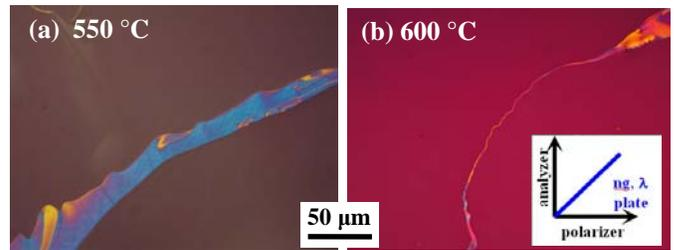
**Fig. 5** OM observation images of cross section vertical to the free surface of the samples heat treated at  $550^\circ\text{C}$  (a) and  $600^\circ\text{C}$  (b).
