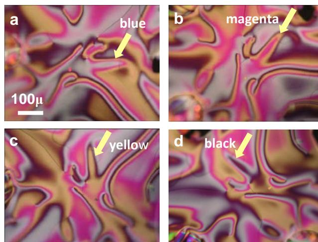
**Fig. 1** Optical microscope images of surface of anisotropic pitch based carbon heat treated at 400°C. These four images are the same place of the surface. The images (b), (c) and (d) are rotated 45°, 90° and 135° counterclockwise, respectively, on the basis of image (a) of 0°. The part of blue color of the arrowed shown in (a) changes to magenta (b), yellow (c) and black (d) with rotations.
