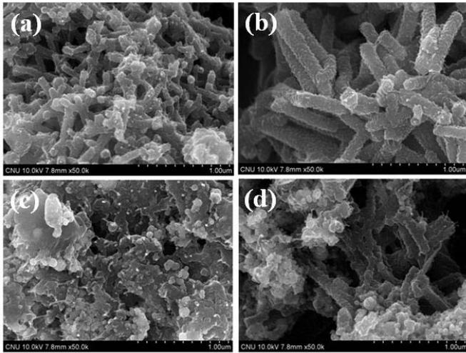
**Fig. 1.** SEM microphotographs of (a) PANI, (b) PC, (c) PF, and (d) PFC.
