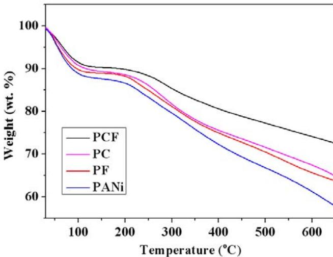
**Fig. 2.** TGA thermograms of various samples.
