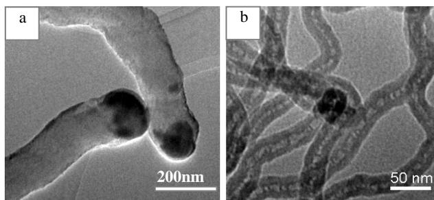
**Fig. 4** HRTEM images of the products prepared at different reaction temperatures using reduced Fe/ABW catalyst by H<sub>2</sub> (a) 600°C; (b) 700°C
