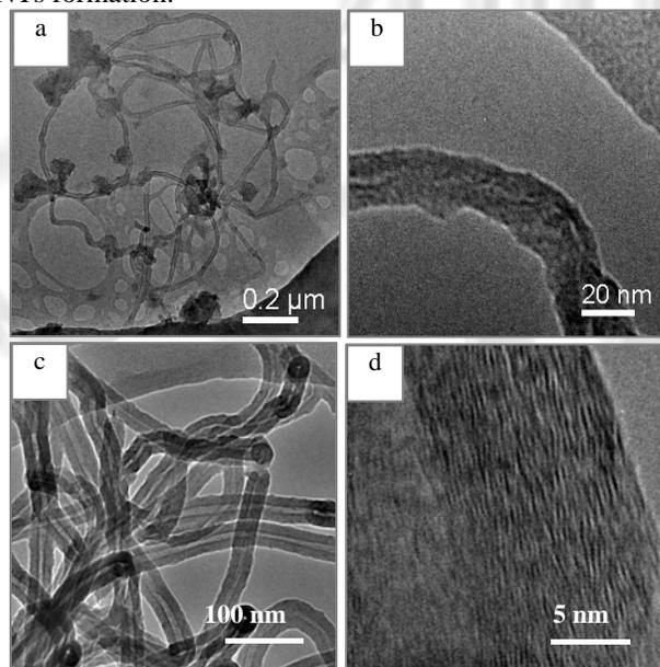
**Fig. 1** HRTEM images of the products prepared at different reaction temperatures using Fe/MCM-41 catalyst. (a) 600 °C; (b) enlarged image of (a); (c) 700 °C; (d) enlarged image of (c)
