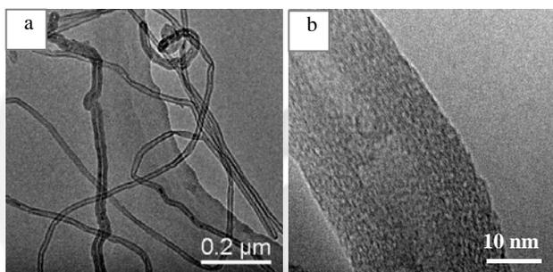
**Fig. 3** HRTEM images of the products prepared at 700°C using Fe/MCM-41 as catalyst without reduction of H<sub>2</sub>. (a) low magnification image; (b) high magnification image
