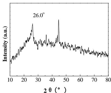
**Fig. 2** XRD patterns of the products prepared at 700°C using Fe/MCM-41 catalyst.
