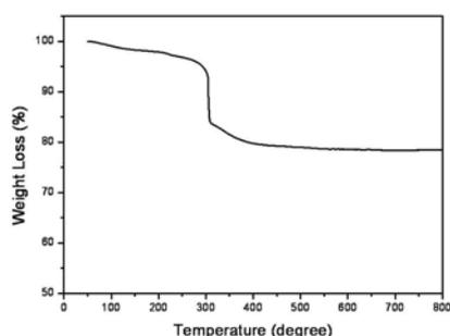
**Fig. 2** Thermogravimetric analyser (TGA) of  $\text{Co}_3\text{O}_4/\text{GNS}$  nanocomposite.
