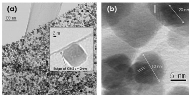
**Fig. 3** TEM image of  $\text{Co}_3\text{O}_4/\text{GNS}$  nanocomposite. (a) low magnification and (b) high magnification.
