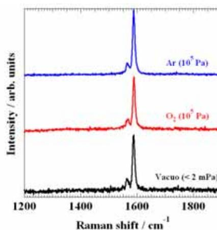
**Fig. 4** SERS spectra of open-SWCNT at high-crystallinity region. The SERS spectra were obtained under Vacuo ( $<2\text{ mPa}$ ), Ar, and  $O_2$  atmospheres.
