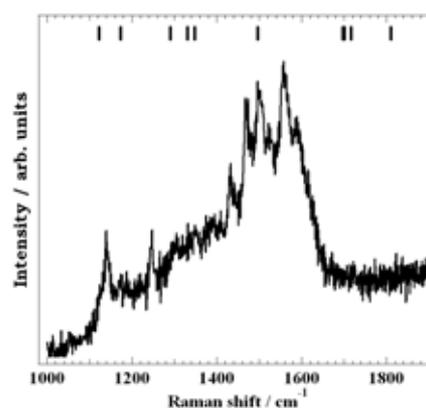
**Fig. 3** SERS spectra of closed-SWCNT at defective region (under 2 mPa). Bars indicate vibrational frequencies associated with a STW defect [7].
