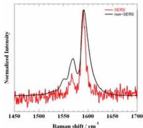
**Fig. 2** SERS spectra of closed-SWCNT at high-crystallinity region (under 2 mPa).
