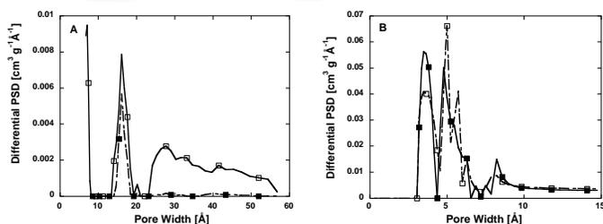
**Fig. 2A:** N<sub>2</sub> isotherm differential PSD obtained by applying DFT method, ■ untreated wheat straw, □ treated wheat straw. **B:** CO<sub>2</sub> isotherm differential PSD obtained by applying DFT method, ■ untreated wheat straw, □ treated wheat straw.
