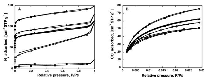
**Fig. 1A:** N<sub>2</sub> adsorption-desorption isotherms of biochars at 77K, ■ untreated wheat straw, □ treated wheat straw, ● pine wood pellets ▲ coastal reed, ◆ Douglas fir pellets.
