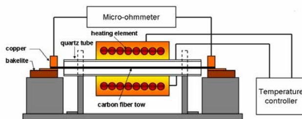
Fig. 1 Experimental setup for the resistance measurement of carbon fibers during oxidation.
