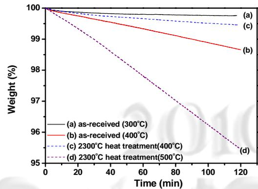
**Fig. 4** Isothermal TGA analyses of as-received and 2300°C heat-treated CFs at different temperatures: (a) as-received CFs, 300°C, (b) as-received CFs, 400°C, (c) 2300°C heat-treated CFs, 400°C and (d) 2300°C heat-treated CFs, 500°C.
