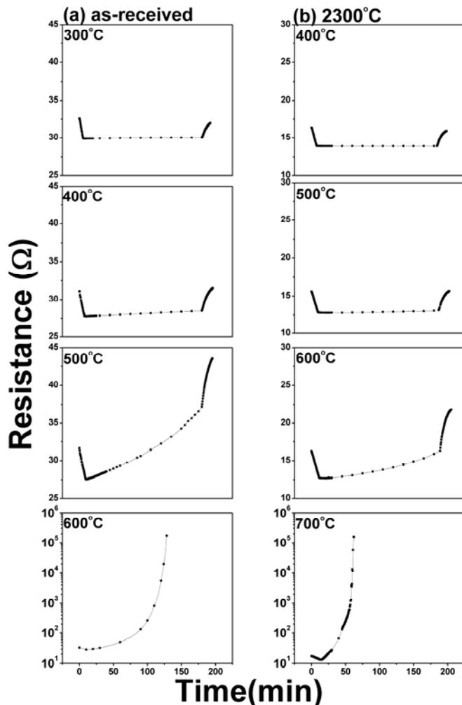
**Fig. 2** Variation in resistance with time during oxidation at different temperatures for: (a) as-received CFs and (b) 2300°C heat-treated CFs.
