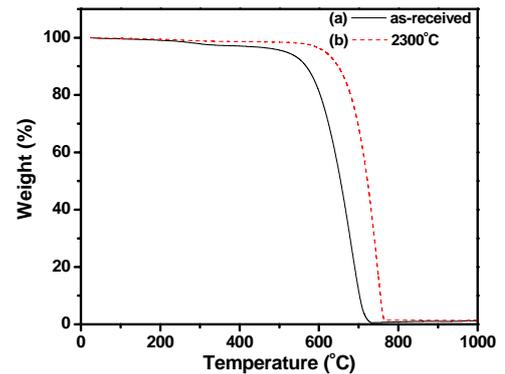
**Fig. 3** Non-isothermal TGA analyses of CFs: (a) as-received CFs and (b) 2300°C heat-treated CFs.
