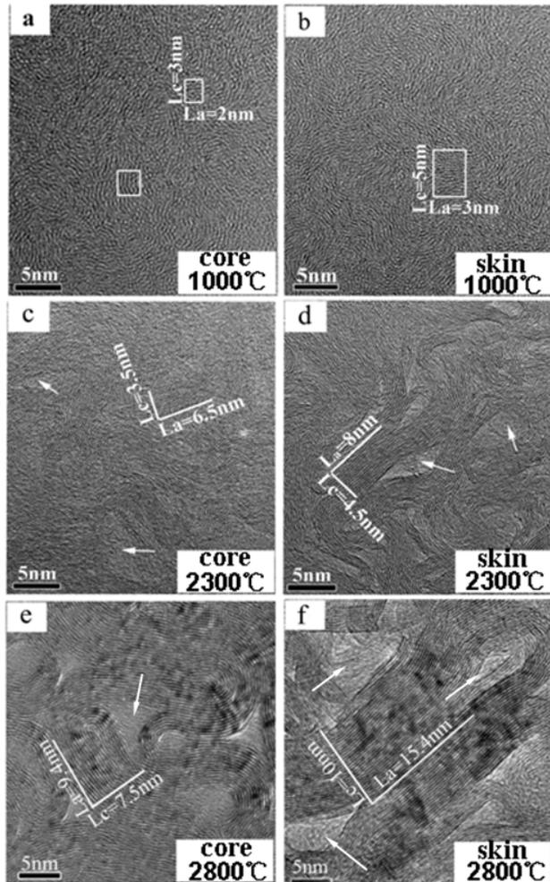
**Fig. 3** HRTEM images of a transversal section, showing the crystallite size and shape in the core and skin regions
