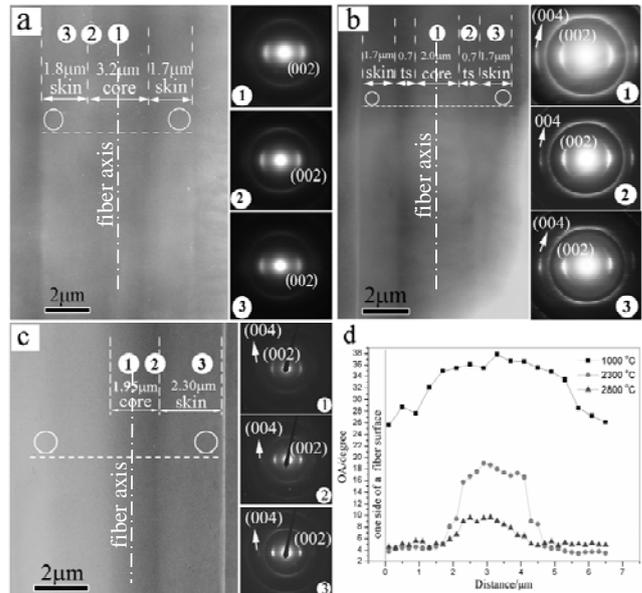
**Fig. 2** Low-magnification TEM micrographs of longitudinal sections of a fiber and their corresponding SAED patterns of the core, intermediate and skin regions after heat treatment at 1000 °C (a), 2300 °C (b) and 2800 °C (c). The OA as a function of the distance from the fiber surface is shown in (d)
