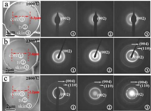
**Fig. 1** Low-magnification TEM micrographs of transversal sections of fibers after heat treatments at 1000 °C (a), 2300 °C (b) and 2800 °C (c) and their corresponding SAED patterns of the core (①), transition (tz) (②) and skin regions (③).
