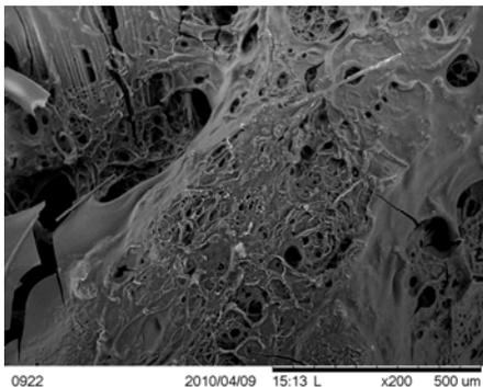
Fig.1 SEM images of a) carbon cloth; b) AC coated carbon cloth; c) AC coated carbon cloth grown with CNTs.
