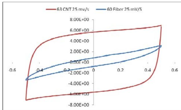
Figure 2. Cyclic voltammograms recorded at 25 mV/s for samples: i) AC formed the carbon cloth (blue drawing); ii) AC formed with CNTs grown on the carbon cloth (red drawing).
