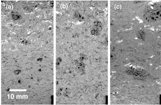
**Fig. 2** Microstructure of the three different coarse grain graphite recipes; trial recipe 1 (a); trial recipe 2 (b); trial recipe 3 (c)
