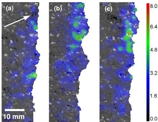
**Fig. 3** Combination of acoustic emission density plots with the CT-analysis; distance of the slice from the sample surface: 25 mm (a); 40 mm (b); 50 mm (c)
