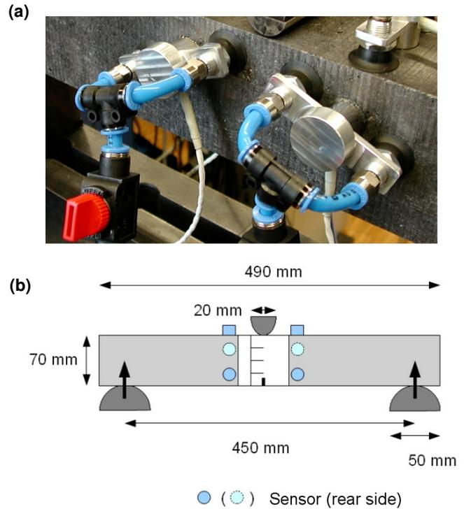
**Fig. 1** Vacuum punch to fix the sensors at the sample surface (a); schematic view of the experimental setup and the used sample size (b)
