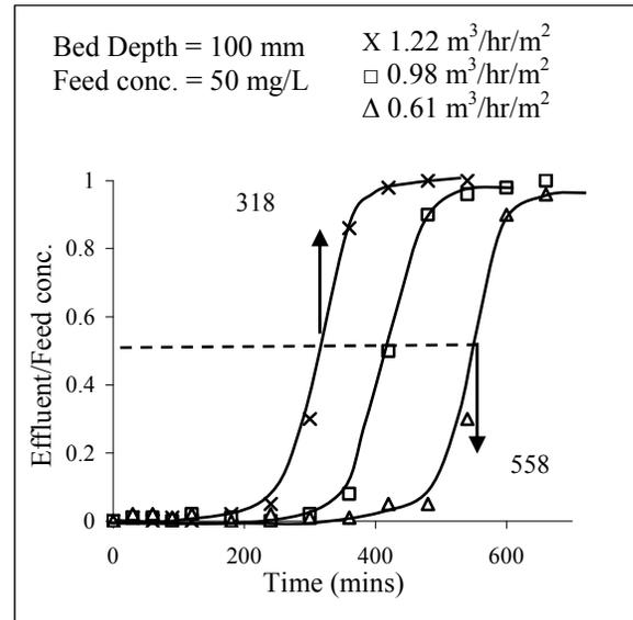
Fig.2 Effect of HLR on breakthrough curve for ACC
