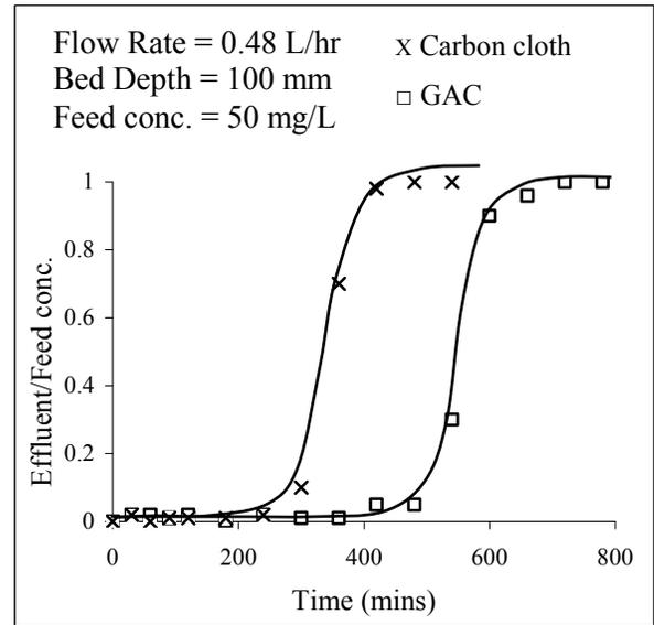
Fig.1 Breakthrough curves of Pb(II) ions on both carbons
