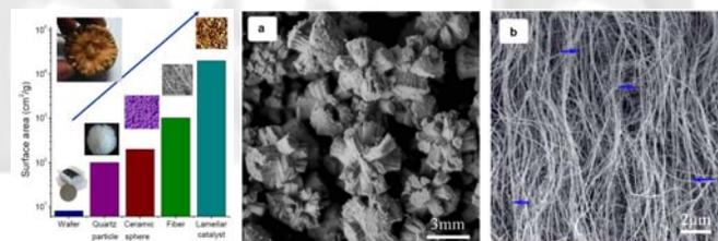
**Fig. 2** Left: To increase the amount of aligned CNT growth, various kinds of particles with high surface area were used as substrate; Right: (a) Large amounts of aligned CNT array grown at 800 °C on sphere; (b) SEM of the aligned CNTs in (a). Type 1 (straight, the arrow pointed CNTs in (b)) and Type 2 (curved) CNTs were shown in the aligned CNT arrays [2].
