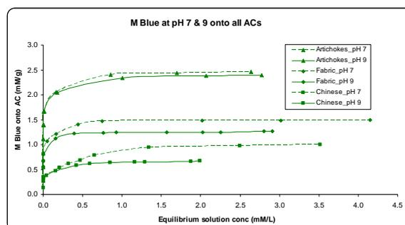
**Fig. 4** Adsorption isotherms at pH 7 & 9 for M Blue on the Fabric, Chinese & Artichokes ACs.
