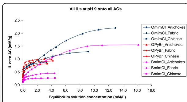
**Fig. 2** Adsorption isotherms at pH 9 for OMImCl, OPyBr & BMImCl on the Fabric, Chinese & Artichokes ACs
