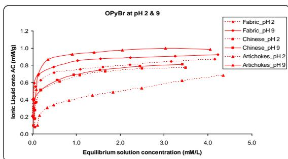
**Fig. 1** Adsorption isotherms at pH 2 & 9 and 25°C for OPyBr on the Fabric, Chinese & Artichokes ACs
