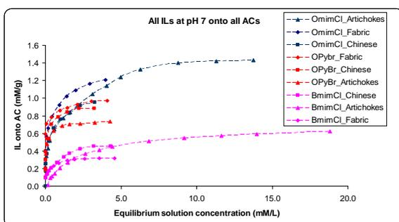
**Fig. 3** Adsorption isotherms at pH 7 and 25°C for OMImCl, OPyBr & BMImCl on the Fabric, Chinese & Artichokes ACs
