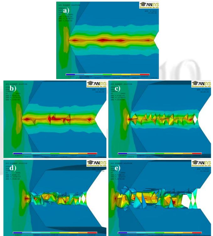
**Fig. 4:** Progressive removal of elements to simulate crack propagation. a) 0 elements removed, b) 22, c) 115, d) 395, e) 932.
