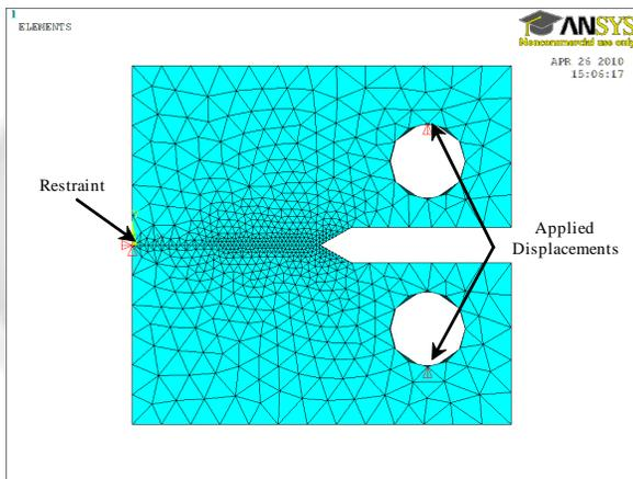
**Fig. 2:** Meshed compact tension model created in ANSYS showing applied restraint and displacements.
