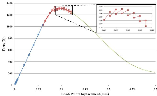
**Fig. 3:** Load-Load point displacement curve generated using the compact tension model and element removal methodology.
