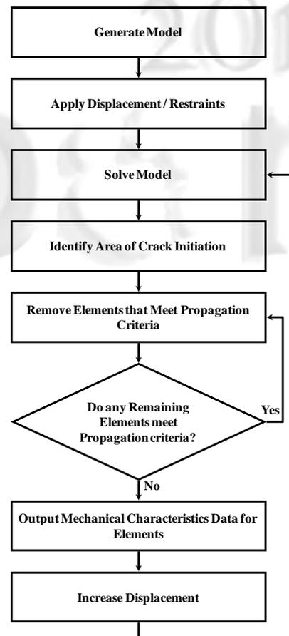
Fig. 1: Outline methodology for progressive removal of elements to simulate crack growth.
