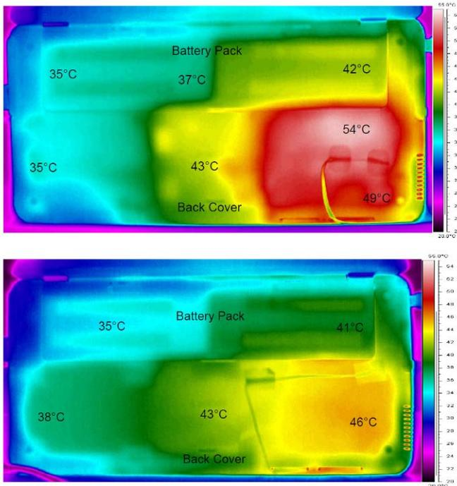
**Fig. 4** IR images of the bottom surface of the Sony VAIO P netbook without (Top) and with (Bottom) a graphite heat spreader.
