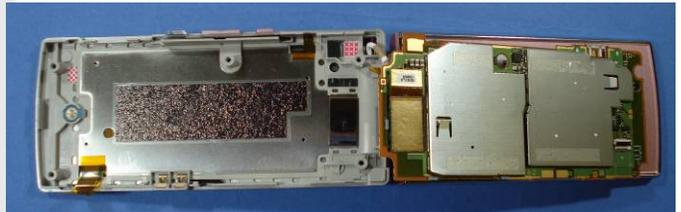
**Fig. 6** A 20µm thick 1500 W/mK graphite heat spreader inside the Sharp SH001 cell phone.
