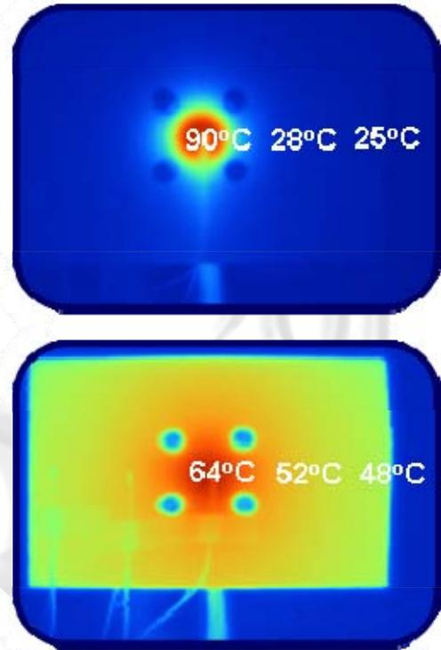
**Fig. 2** IR images of a bare ABS plastic case with a 0.8W heat source attached (Top) and the same case with a 110µm thick 400 W/mK graphite heat spreader and 3.3W heat source attached (Bottom)
