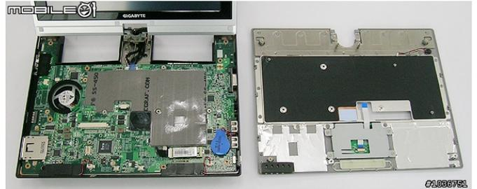
**Fig. 5** The application of a graphite heat spreader to cool an Intel Atom Processor and Chipset in the Gigabyte M912V netbook.
