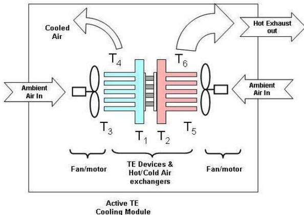
Fig. 1 Schematic diagram for thermoelectric cooler system
