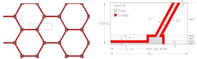
**Fig. 2** Hexagonal mesh of coated foam with unit cell
