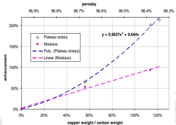
**Fig. 5** Increase of mechanical properties with copper coating
