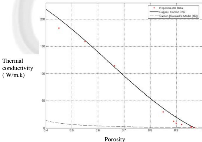
**Fig. 4** Thermal conductivity versus porosity for coated foam
