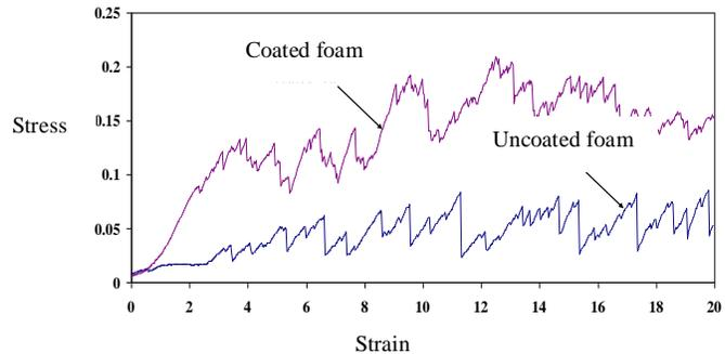
**Fig. 3** Stress-Strain curve for uncoated and coated foam
