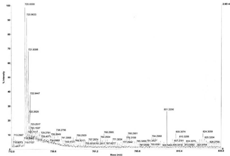
Fig.2. MALDI-TOF mass spectra of fullerene derivatives for the Zn-containing fullerene.
