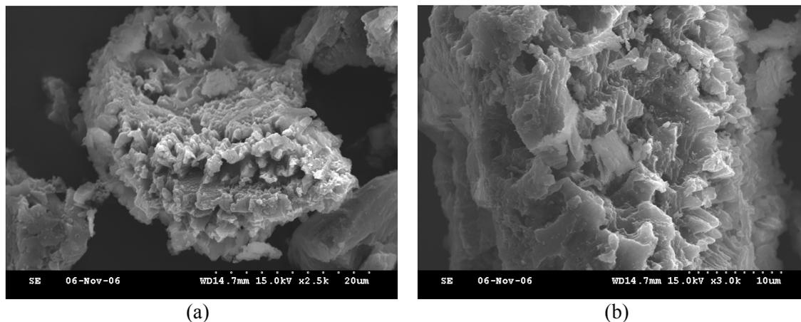
Fig. 1. SEM micrographs of pristine fullerene and fullerene derivatives; (a) and (b) : Zn-containing fullerene.
