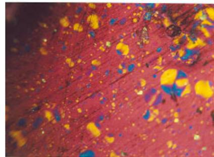
**Figure 2.** M2 pitch heated 425 for 1,2, and 3 hrs.
