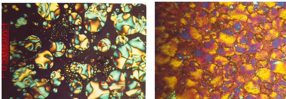
**Figure 1.** Optical micrographs of M1 pitch after 425°C for 1 hr and for 3 hrs.
