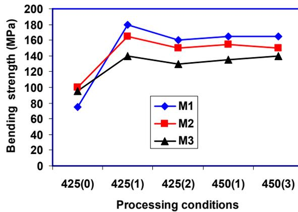
Figure 7: Variation in bending strength with processing stages of mesophase formation in composites.
