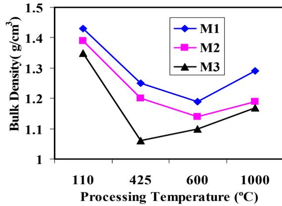
**Figure 4:** Bulk density with processing stage of composites with different pitches (at 425°C for 1hr.)
