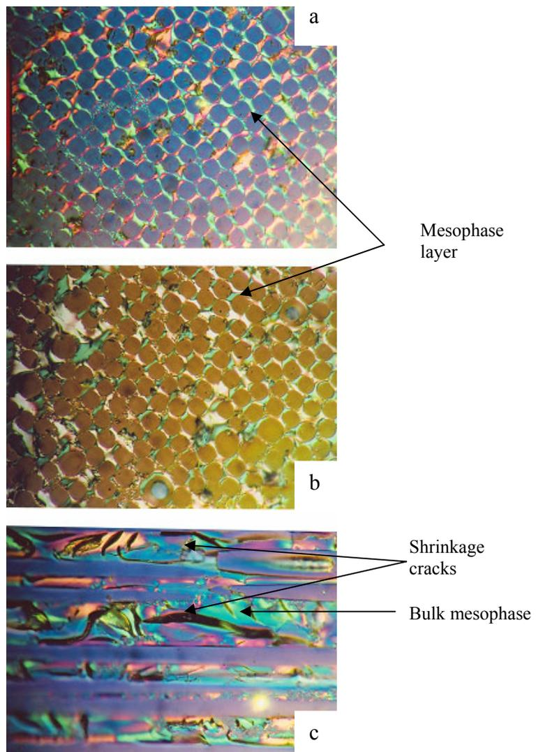
**Figure 5:** Optical micrographs of M1 pitch based C/C composites
