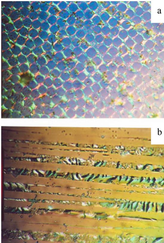
Figure6. Optical micrographs of M3 pitch based C/C composites
