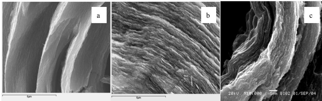
**Figure 3.** Scanning electron micrographs of fracture surfaces of pyrocarbon matrix layers of the felts obtained in the three-point bending test; (a) feltI, (b) feltII, (c) feltIII.
