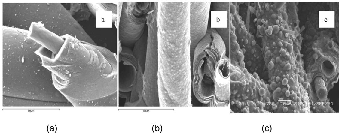
**Figure 4.** Scanning electron micrographs of deposition surface of pyrocarbon around carbon fiber in C/C composites; (a) feltI, (b) feltII, (c) feltIII.
