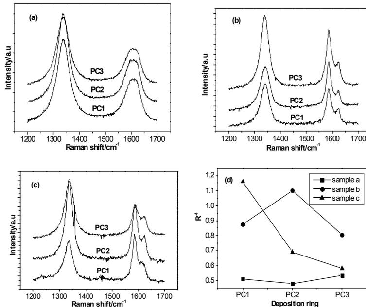
**Figure 2.** Raman spectras of pyrolytic carbon of different deposition stage around a fibre; (a) feltI, (b)feltII, (c) feltIII, (d) changes of Raman parameter  $R^{-1}$  of samples (a), (b), (c); PC-pyrocarbon.
