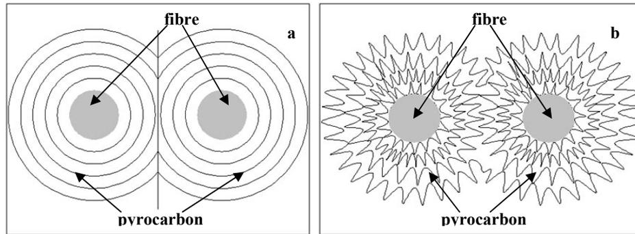
**Figure 5.** Two typical growth model pyrolytic carbon by CVI
