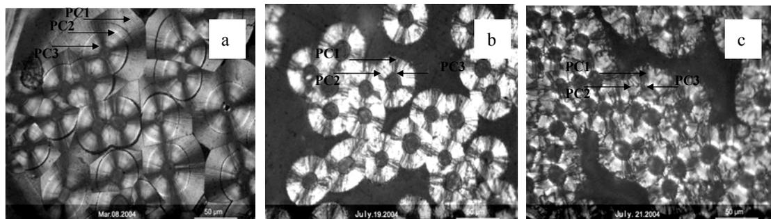
**Figure 1.** Three typical polarized optical micrographs of samples from the infiltrations; (a) feltI, (b)feltII, (c) feltIII, the samples (a), (b), (c) are deposited at a pressure of 4kPa and temperatures of 1220K, 1270K, 1320K, respectively.
