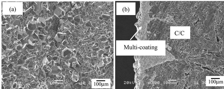
Fig 2. SEM micrographs of the SiC/W-Mo-Si coated C/C composites obtained by the two-step pack cementation (a) surface; (b) cross-section
