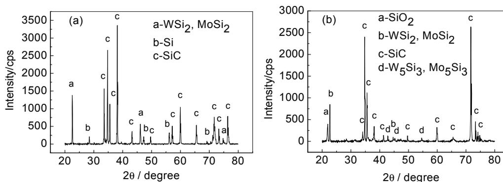
Fig 3. X-ray patterns of the surface of the SiC/W-Mo-Si coating prepared by the two-step pack cementation (a) before oxidation; (b) after oxidation in air at 1773 K for 200 h.
