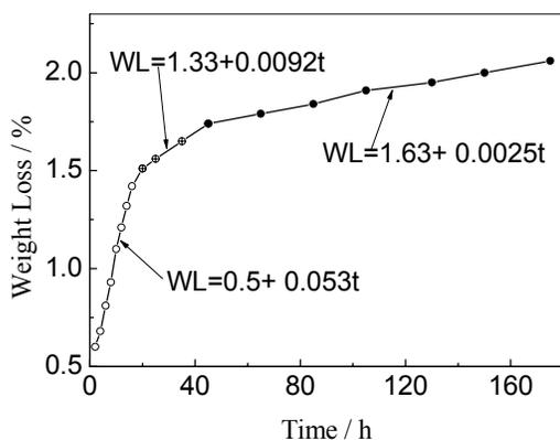
Fig 4. Isothermal oxidation curve of the SiC/W-Mo-Si coated C/C composites in air at 1773K
