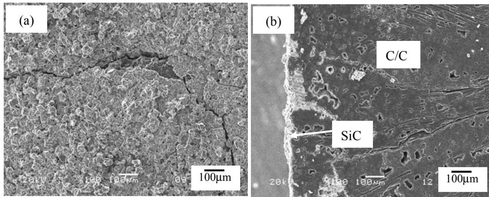
Fig 1. SEM micrographs of the SiC coating prepared by the first-step pack cementation (a) surface; (b) cross-section
