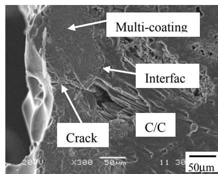
Fig 5. Cross-section SEM micrograph of the multi-coating coated C/C composites after oxidation in air at 1773K for 200h.
