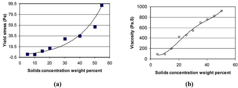
**Figure10.** a) Yield stress and b) Viscosity variation with solids concentration for carbon black suspensions (At pH 11.5)
