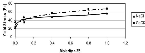
**Figure9.** Effect of increasing conc. of monovalent and divalent cation additions on the yield stress of a 20w/o carbon black suspension (pH=11.5)
