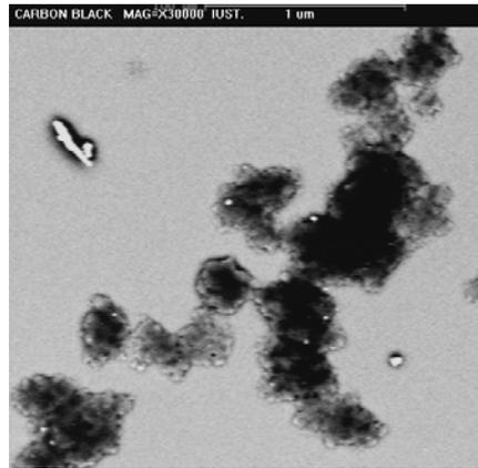
**Figure4.** SEM micrographs of carbon black
