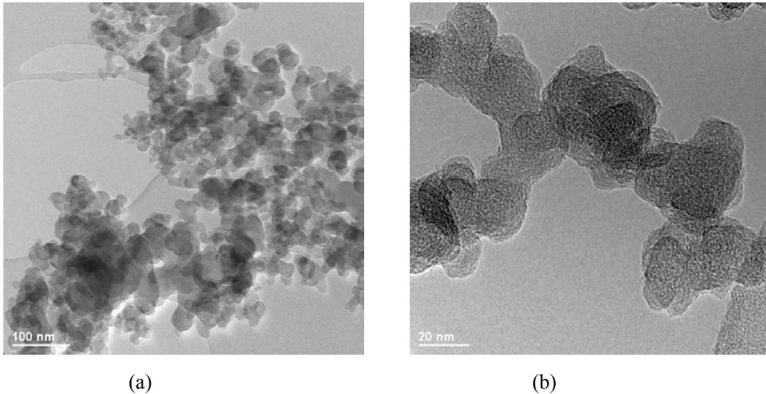
**Figure5.** a) TEM, and b) HRTEM micrographs of carbon black
