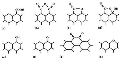
**Figure1.** Possible structure of surface oxygen groups (see text)
