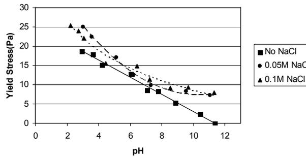
**Figure7.** Variation in Yield stress with pH and Sodium Ion concentration for a 20w/o carbon black suspension
