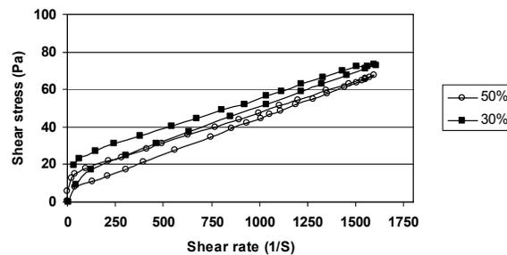
**Figure11.** Variation in flow behavior with increasing solids concentration of carbon black suspensions
