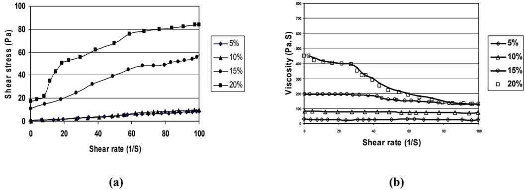
**Figure6.** - Variation in a) Shear Stress and b) Viscosity with Shear rate for 5-20 w/o carbon black suspensions
