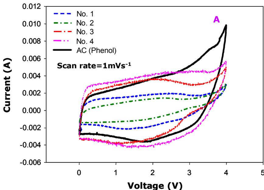
Fig. 2 Cyclic-voltammograms (CVs) of the silk carbon-based ACs and the phenolic resin-based AC as a standard at the sweep rate of  $1\text{mV}/\text{s}$  in the two-electrode system with symmetric configuration.
