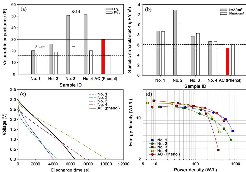
Figure 1. The capacitor properties of silk carbon-based ACs and the standard; the gravimetric and volumetric capacitances (F/g, F/cc) (a) and the capacitance per unit area (μF/cm<sup>2</sup>) (b) at 1 and 10 mA/cm<sup>2</sup> of the discharge current densities, the discharge profiles at the 1mA/cm<sup>2</sup> of the current density (c), and the Ragone plots based on the volumetric dimension (d). All data were obtained by charging up to 3.0 V.
