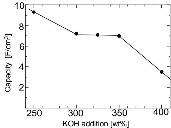
Fig.3 Change in electric double layer capacity of KOH activation
