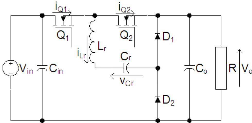
Figure 5. An electronic circuit called switched-capacitor under test
