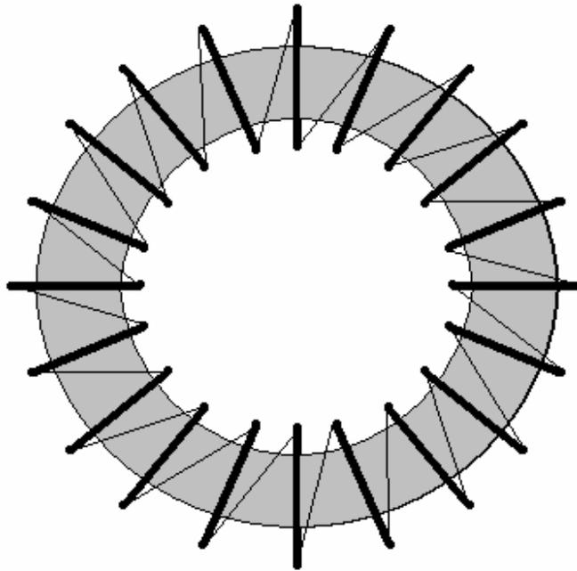
**Figure 2.** The construction of the ring core inductor where grey colour is embedded on the PCB. The winding is plated on the PCB and shown with thick black line for upper conductor wire and thin black wire for underneath wire.
