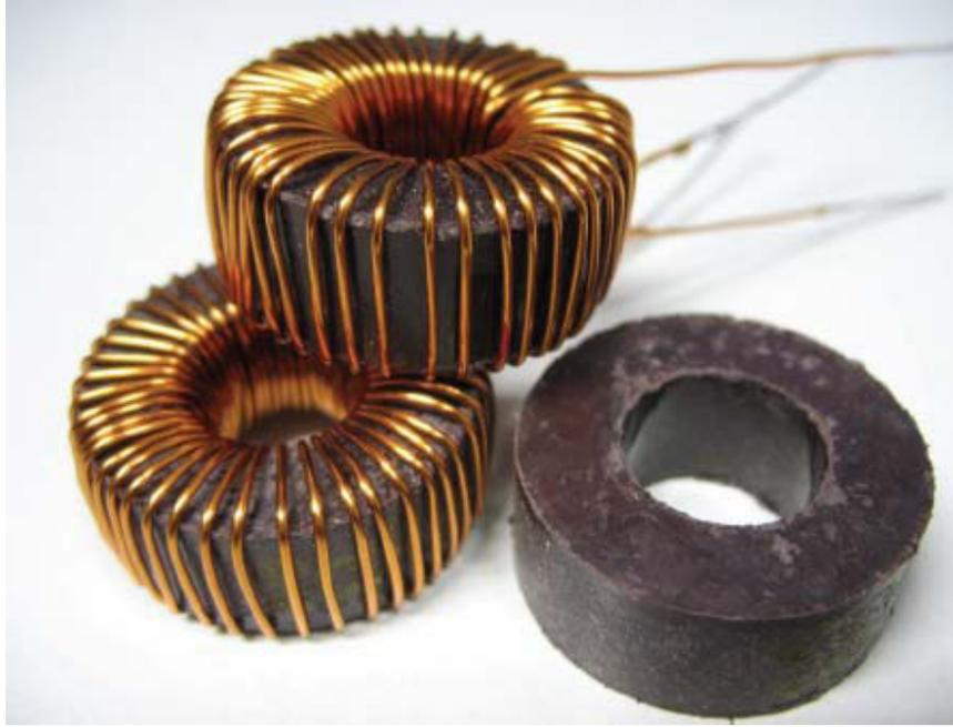
**Figure 7.** The composite using 10%PE-10%PMMA-80%NiZn to construct a sample
