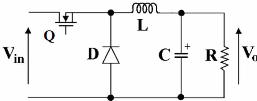
Figure 6. An electronic circuit Buck converter under test
