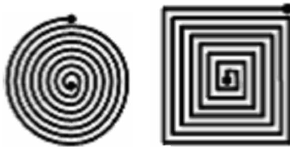
**Figure 3.** Two types of structure of the spiral core inductor using air-core and the wing is just painted on the circuit board.
