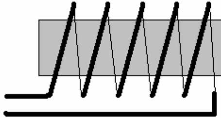
**Figure 1.** The construction of the solenoidal inductor where grey colour is embedded on the PCB. The winding is plated on the PCB and shown with thick black line for upper conductor wire and thin black wire for underneath wire.
