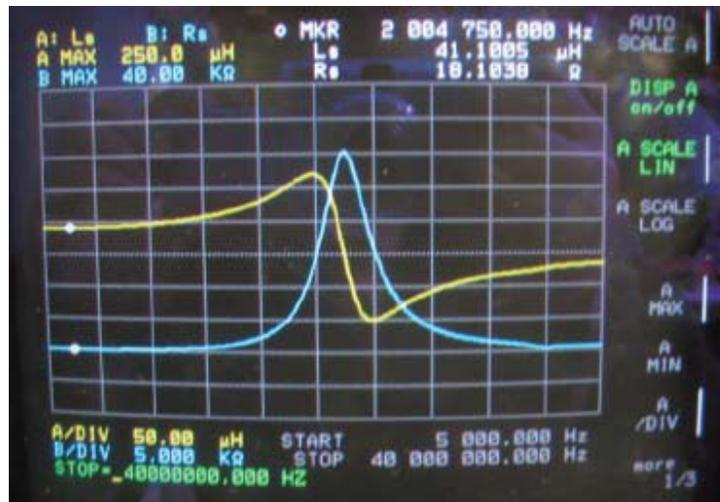
**Figure 8.** Measured variation of the resistance and inductance of the inductor.
