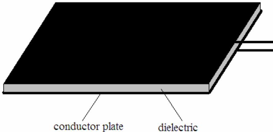
Figure 4. The construction of the capacitor
