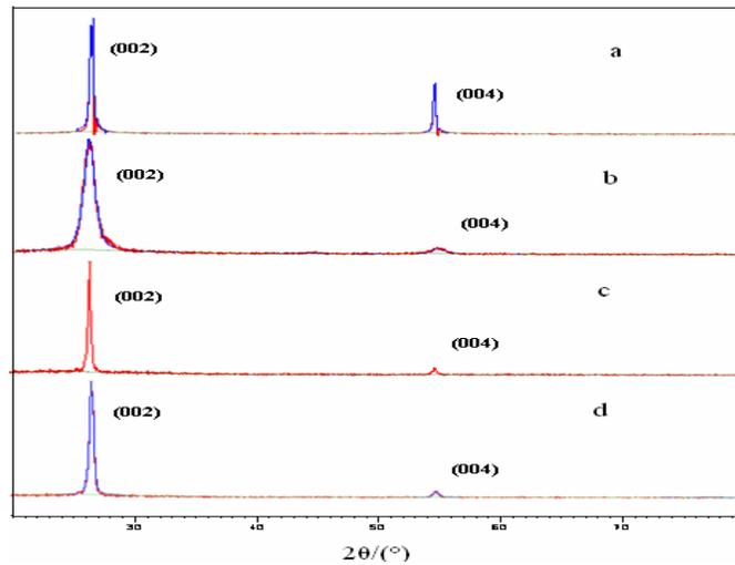
**Fig 3-7.** XRD patterns(a Flake graphite, b Graphite oxide, c Expanded graphite compressed by 5MP, d
