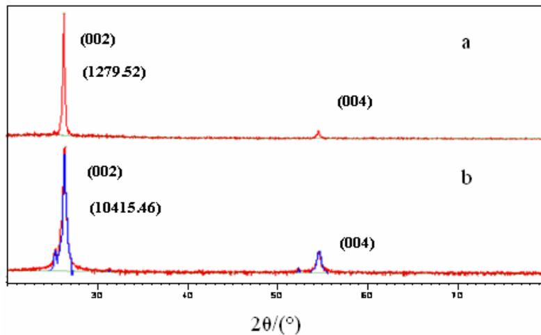
**Fig 3-8.** XRD patterns of expanded graphite compressed by different methods
