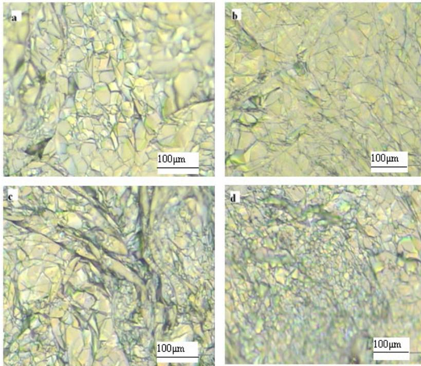
**Fig 3-1.** The phase diagram of expanded graphite at different specification (500×) (a,b Expanded graphite of 32 mesh; c Expanded graphite of 50 mesh; d Expanded graphite of 100 mesh)
