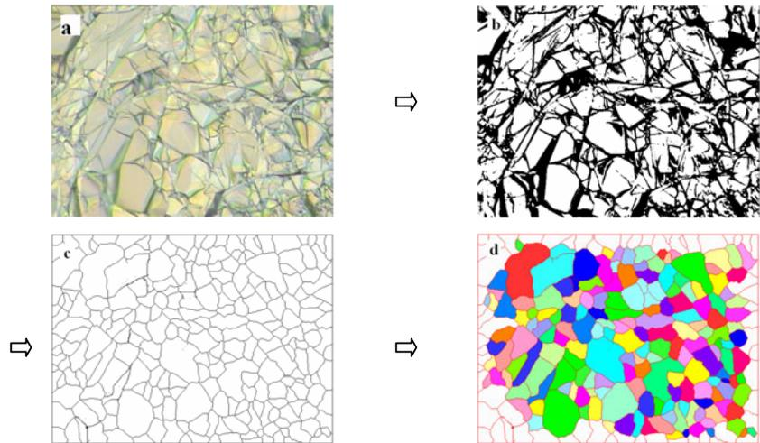
**Fig 3-3** Procedure images of grain-size analysis (a original image ; b threshold division ; c crystal boundary reconstruction ;d Rating (area method)
