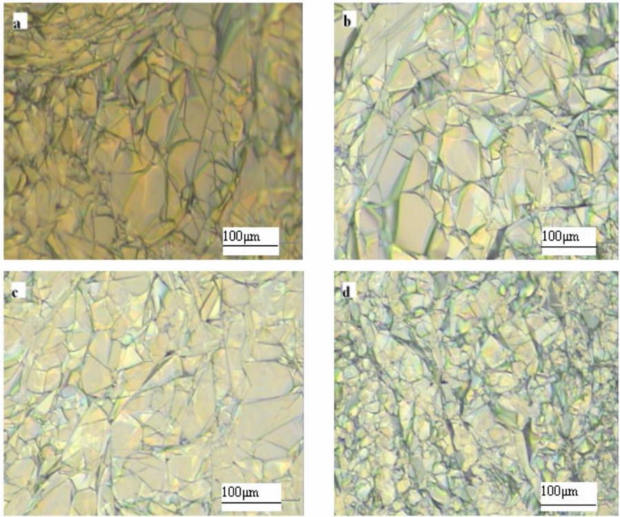
**Fig 3-2.** the phase diagram of the expanded graphite when the quantity of  $\text{KMnO}_4$  is different (500 $\times$ ) (a addition quality is 0.1g;b addition quality is 0.2g;c addition quality is 0.3g;d addition quality is 0.6g)
