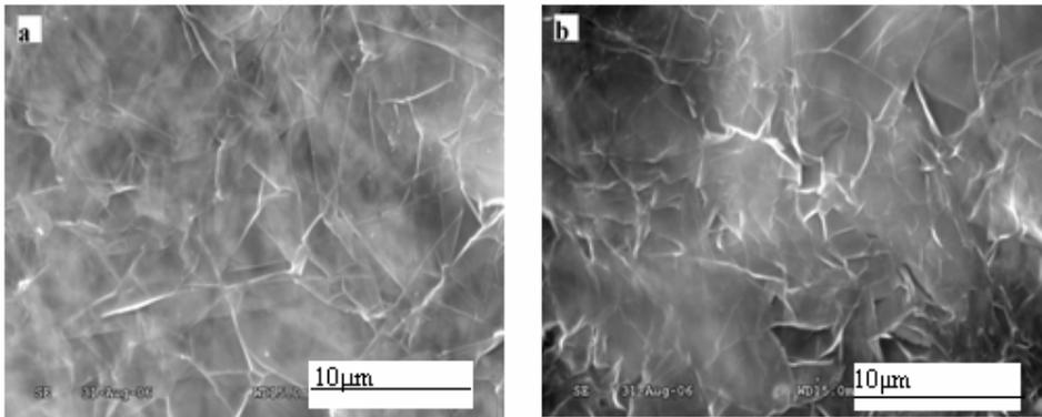
**Fig 3-6.** SEM photos of compressed expanded graphite ( a 4000×; b 5000× )
