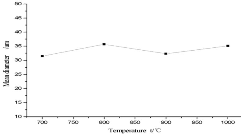
**Fig 3-5. The mean diameter of the expanded graphite under different temperature**
