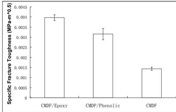
**Figure 13.** Change of specific fracture toughness after resin infusion.
