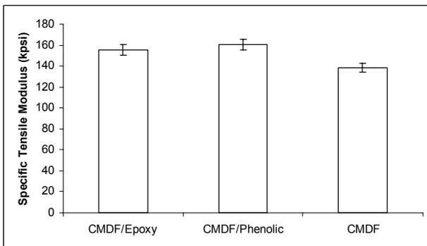
**Figure 12.** Change of specific tensile modulus after resin infusion.
