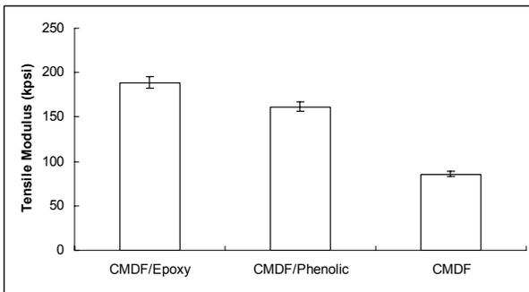
**Figure 5.** Change of tensile modulus after resin infusion.
