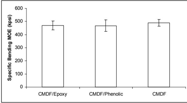
**Figure 9.** Change of specific bending MOE after resin infusion.
