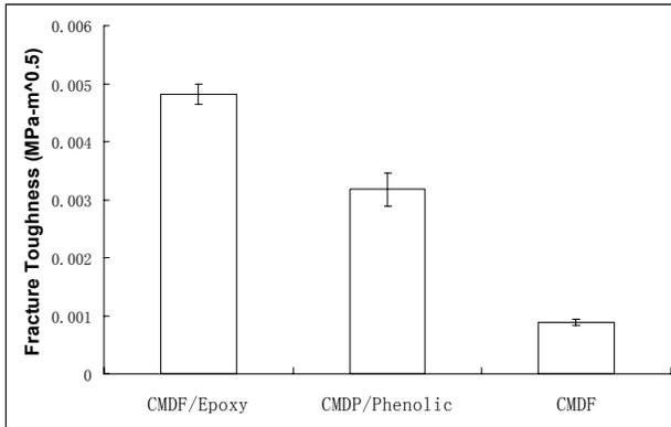
**Figure 8.** Change of plane-strain fracture toughness after resin infusion.
