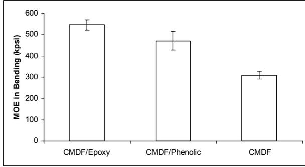
**Figure 7.** Change of bending MOE after resin infusion.
