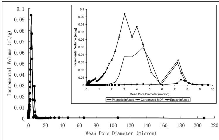
**Figure 2.** Pore size and distribution before and after resin infusion.
