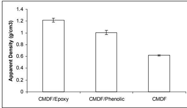
**Figure 1.** Change of apparent density after resin infusion.
