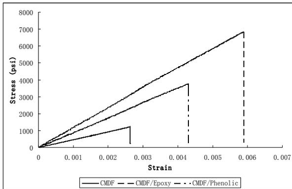
**Figure 3.** Typical stress-strain profiles of CMDF, CMDF/Epoxy composite, and CMDF/Phenolic composite.
