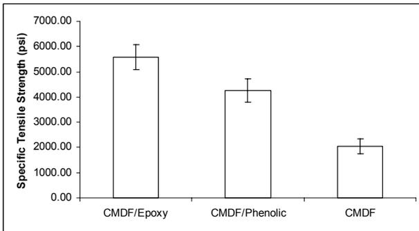
**Figure 11.** Change of specific tensile strength after resin infusion.
