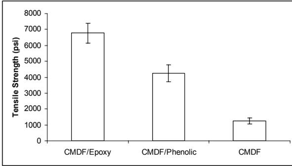
**Figure 4.** Change of tensile strength after resin infusion.
