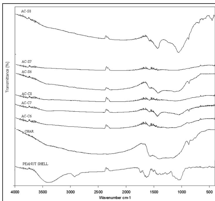
**Figure 3.** FT-IR spectra of produced char and activated carbons
