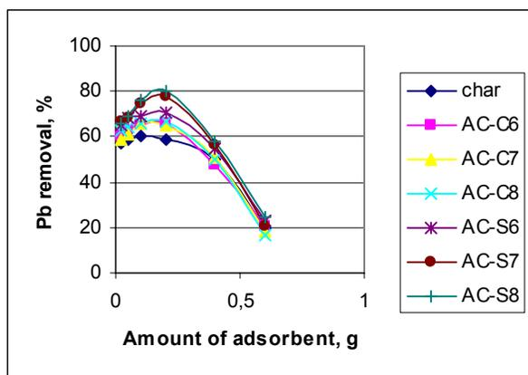
Figure 4. Effect of adsorbent amount on Pb<sup>2+</sup> adsorption
