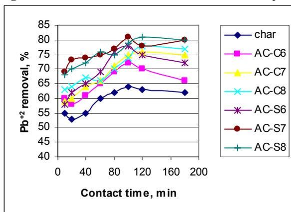
Figure 6. Effect of contact time on Pb<sup>2+</sup> adsorption
