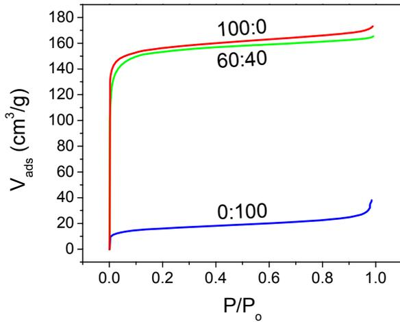
**Figure 8.** Nitrogen adsorption isotherms for carbons made from pure crystalline cellulose (100:0), phenolic resin (0:100) and a blend of the two (60:40).
