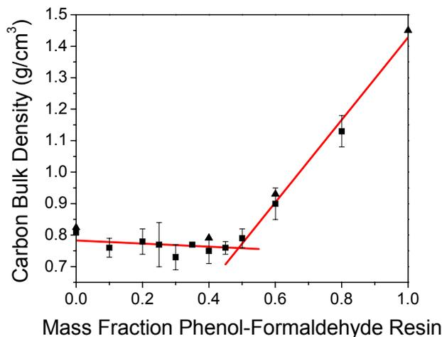
**Figure 6.** Bulk density of carbon monoliths made from crystalline cellulose – phenolic resin blends.
