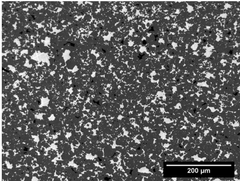
**Figure 9.** Optical micrograph of polished cross-section of siliconized carbon. Black regions are C, gray are SiC, and white are Si.
