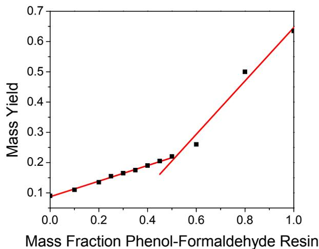
**Figure 5.** Mass yield of carbonized crystalline cellulose – phenolic resin precursor blends.
