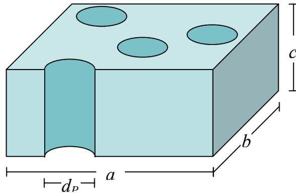
**Figure 2.** Schematic of porous carbon substrate of length,  $a$ , depth,  $b$ , height,  $c$ , and pore diameter  $d_p$ .
