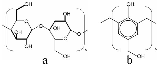
**Figure 3.** Chemical structures of crystalline cellulose (a) and phenolic resin (b).
