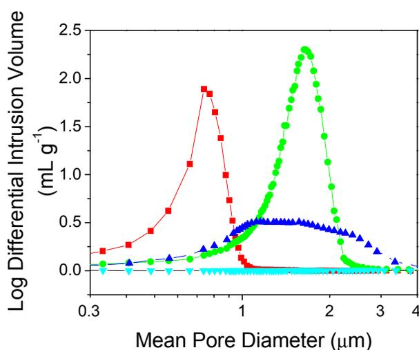
**Figure 7.** Pore size distribution of porous carbons created from various precursor blends.
