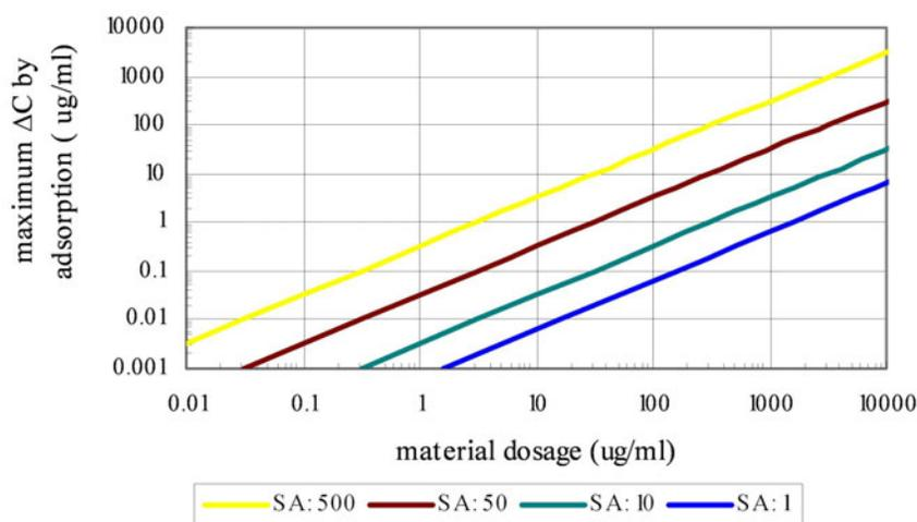
Fig. 1: Potential for nanomaterials to alter biological fluid phases by adsorption. Plot gives maximum concentration change by adsorption at monolayer coverage for materials with various surface area (SA: m<sup>2</sup>/g) and dose. This example calculation is for typical of small (non-macromolecular) biomolecular solutes, assuming 1nm<sup>2</sup> surface area/ molecular and only monolayer physical adsorption
